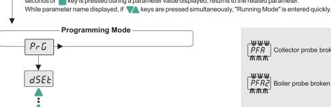
By pressing these two keys simultaneously and hold down for 2 seconds, LP 1 message appears and user menu is entered and name of the first parameter will be displayed
