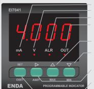
mA LED : If input type is selected as 0-20mA or 4-20mA, mA LED lights up. V LED
