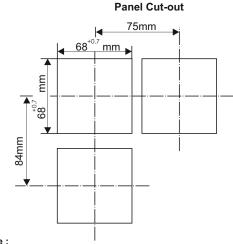
1) Panel thickness should be maximum 10mm.
