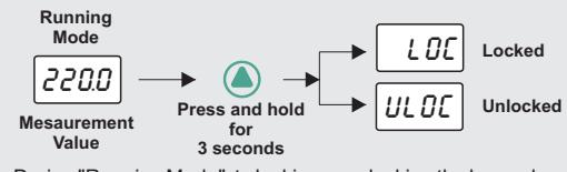
During "Running Mode", to locking or unlocking the keypad, key is pressed for 3 seconds. *LOC* or *ULOC* message will appears for valid status.
