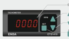
(1) Indicates measured value and set values in "Running Mode". Indicates the parameters and names in "Programming Mode".
