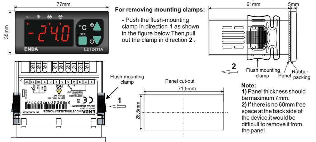
For removing mounting clamps:
