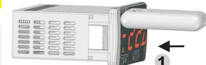
Move ENDAKEY-RF towards the top left of the device in direction 1
