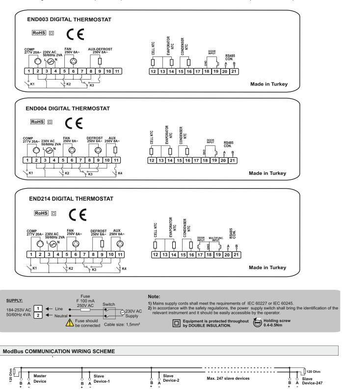
The start and end of the communication line must be terminated with a 120 Ohm resistor.
