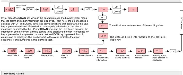
W W W UP UP value → DOWN)-SET 🕨 149 SET - 150 РЬ2 rLS 0 DOWN DOWN If you press the DOWN key while in the operation mode (no key lock), enter menu that the alarm and other information are displayed. From here, the r L 5 message is selected with the UP and DOWN keys. When the SET key is pressed and the UP and DOWN keys are set to "149 " password and the SET key is pressed, the message
