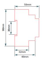
: 3 Phase and 1 Neutral; 230 Vac) : (0.5 – 1.5) x Un ; (Un nominal voltage) : 50/60 Hz : Please refer to table : Please refer to table : Below Un x 0.65 and above Un x 1.35 : 500 msec : Max. 5 A / 240 VAC : < 8 VA : IP20 : IP00 : -5°C....+50°C : To connection rail in electrical panel : 35x90x58 mm
